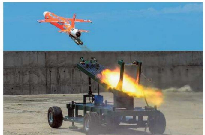
Defence Research and Development Organisation (DRDO) on Wednesday successfully flight-tested ABHYAS, a high-speed expendable aerial target – used as an aerial target for evaluation of missile systems at low altitude – at the integrated test range in Chandipur off the coast of Odisha. Defence Minister Rajnath Singh congratulated DRDO and the armed forces, and said the system will meet requirements of the forces
